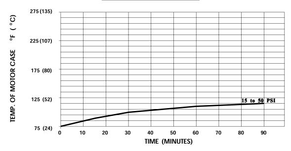
THIS GRAPH IS FOR USE AS A DESIGN GUIDE. IT IS BASED ON RUNNING CONTINUOUSLY WITH AN AMBIENT TEMPERATURE OF 75° F IN STILL AIR. THE THERMAL BREAKER WILL OPEN WHEN THE CASE TEMPERATURE REACHES  $280^\circ$  F.
